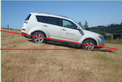
Slope greater than 7 degrees (actual slope of 14 degrees)
